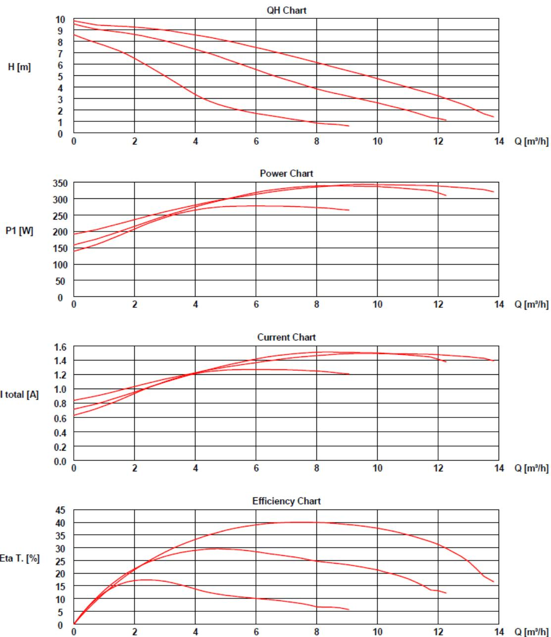
Performance test based on standard ISO 9906 with pre-pressure 2.0bar and liquid temperature 20°C. /性能测试依标准 ISO 9906, 系统初始压力 2.0bar, 液体温度 20°C .
